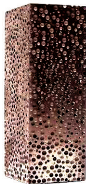
North Carolina State University has developed a porous steel that offers high protection but is much more lightweight.
